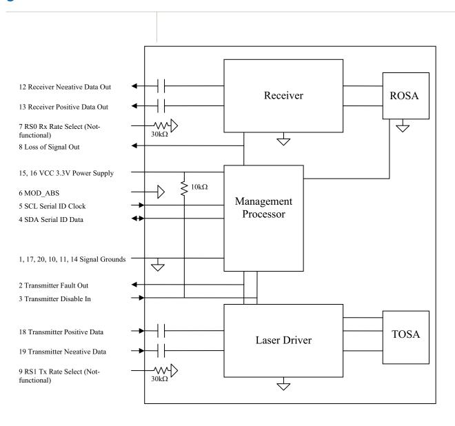
Figure 1 SFP+ optical transceiver functional block diagram
