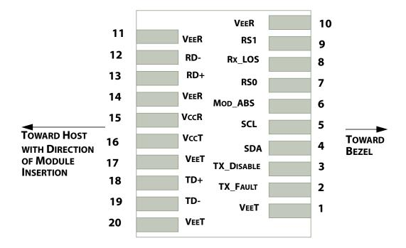
Figure 3 Host PCB SFP+ Pad assignment top view
